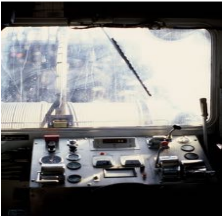
The Winch Driver's panel and the logging cable (note the oily window).
